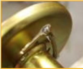
Swaged ball fitting allows for easy installation of wire rope assemblies. Four drum wraps required for proper operation.
